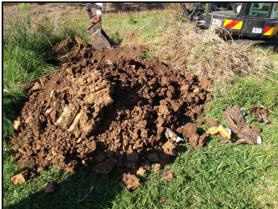
Photo 6: Facing south – Test pit 2 (TP2) example of waste materials buried in the soil mounds. Riparian zone is in the background.
