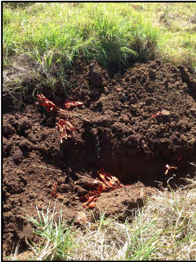
Photo 5: Test pit 6B (TP6B) where asbestos was detected. There were no obvious potential asbestos containing materials present such as fibro sheeting. Other anthropogenic waste materials are present.
